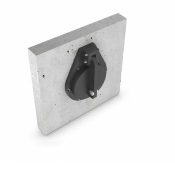
Wall mounted HDPE Flap Valve ATK0100G Stainless steel fixings. Opening Ø100 mm - Ø2000 mm. 5 M.w.c. On seating.
